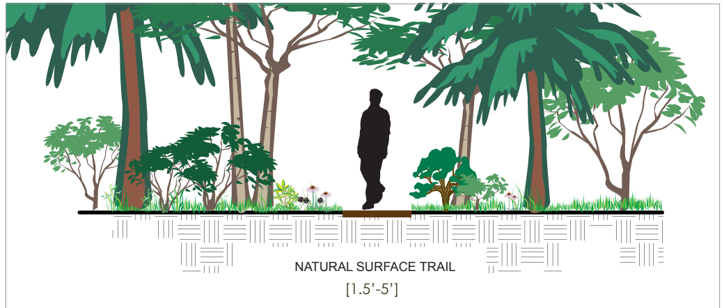
Right: Typical natural surface trail section
